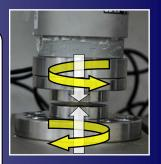
Yield Torque: 37.2 N-m (329 in-lbs) Peak Torque: 47.7 N-m (422 in-lbs)
